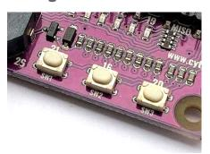
3 units of programmable push button are included in the Maker pHAT. To utilize it, user need to configure push button GPIO as input pullup.
