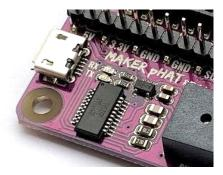
Serial remote is a helpful tool to get started with Raspberry Pi. Luckily, Maker pHAT comes with USB to Serial module for this purpose. It is connected to Raspberry Pi's UART pin (RX and TX). Please refer to Getting Started section for more detail.
