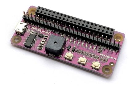
No worry about short circuit when you stack the Maker pHAT Rev1.10 on the <u>Raspberry Pi Zero WH</u>.
