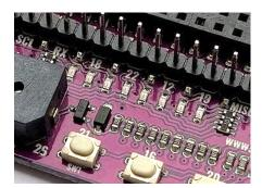
8 LEDs is connected to GPIO 17, 18, 27, 22, 25, 12, 13 and 19. Those LED can be controlled as an output or can be act as an input (signal monitoring). In other words, GPIO that connected to the LED, can be configured as output, input and input pull up.
