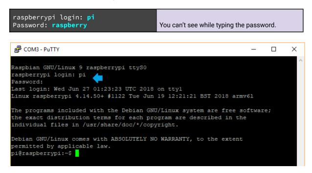
So far, you're able to access Raspberry Pi through serial remote (Maker pHAT). We will further guide you until we can remote using <u>VNC Viewer</u> (Virtual Network Computing).
