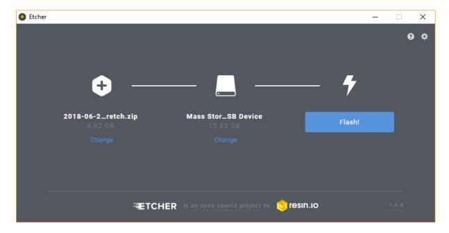
After done flashing, take the <u>SD card</u> out and insert back to your laptop. Open <u>SD card</u> directory (e.g. D:/boot) and open **config.txt** file. Put **enable\_uart=1** at the bottom of the line. Save and eject the <u>SD card</u>. Then insert the <u>SD card</u> into <u>Raspberry Pi Zero WH</u>.
